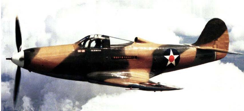
With its 37-mm cannon and six machine guns the P-39 packed a big punch and was the best plane available to rush into service. The P-39's being readied for the 35<sup>th</sup> Squadron had originally been
